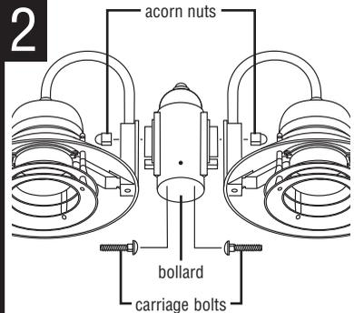
Attach each assembly from Figure 1 to bollard base with carriage bolt, and plastic acorn nut.
