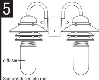
Screw diffuser into roof.
