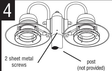
Position the fixture over the post as shown. Fasten with screws at holes in post collar by drilling holes at same location through the post and securing with screws.
