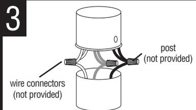
Connect the wires. Note: Attach black fixture wires to black supply wire, white fixture wires to white supply wire. Do not mix them up. Use wire connectors (not provided). Connect bare fixture ground wires to ground from outlet box. NEVER CONNECT GROUND WIRE TO BLACK OR WHITE POWER SUPPLY WIRES.
