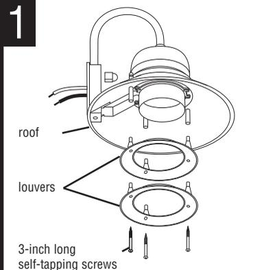
Attach louvers to roof as shown.
