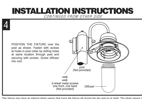
This fixture may have an integral photo sensor that turns the fixture off during the day and on at night. The photo sensor is not adjustable. The fixture could possibly cycle on and off due to light reflected from nearby surfaces into the photo sensor. If cycling occurs, remove the photo sensor nut and install the swivel hood and base.
