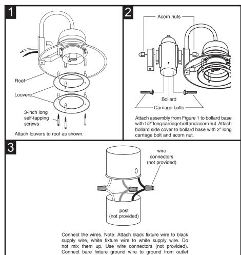
box. NEVER CONNECT GROUND WIRE TO BLACK OR WHITE POWER SUPPLY WIRES.
