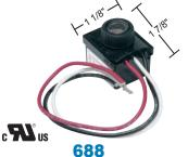
120V Button Photo Control 11/16" Dia. mounting hole required Up to 300W Inc., 54W LED 39W Fluor., 100W H.I.D. SPECIFY: Black
