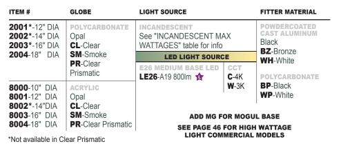
RECOMMENDED EQUIVALENT **INCANDESCENT MAX WATTAGES** POLYCARBONATE **ACRYLIC** DIA 10" 75W 12" 100W 100W 14" 150W 150W 16" 150W 150W 18" 150W 150W
