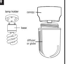
Align and insert the round ended pins on the bottom of the self ballasted lamp into the circular opening in the lamp holder key hole slots. Grasp the base and rotate clockwise. Use lamp type specified on the fixture. Thread diffuser into canopy.
