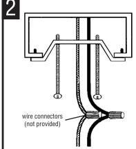
CONNECT THE WIRES. NOTE: Attach black fixture wire to black supply wire, white fixture wire to white supply wire. Do not mix them up. Use approved wire connectors (not provided).
