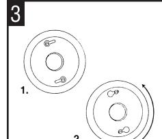
INSTALL canopy to ceiling. Push fixture wire into outlet box. Align head of mounting screws with large end of key hole slots, push canopy towards ceiling. Rotate canopy counterclockwise and tighten screws.
