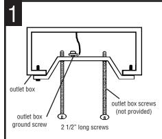
Insert outlet box screws (not provided) through oval slots in cross bar and attach to outlet box. Screw 2 1/2" long screws into the outer most threaded holes.
