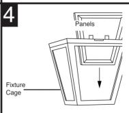
Install plastic panels, textured or beveled side out, by sliding panels down cage in slots on inside of cage. Make sure panels are all the way down in seats in cage.
