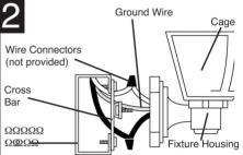
CONNECT THE WIRES. NOTE: Attach black fixture wire to black supply wire, white fixture wire to white supply wire. Do not mix them up. Use approved electrical tape or connectors (not provided). Connect bare fixture ground wire to ground wire from outlet box. NEVER CONNECT GROUND WIRE TO BLACK OR WHITE POWER SUPPLY WIRES.
