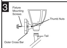
**POSITION THE FIXTURE HOUSING** over the fixture mounting screws and secure in place with thumb nuts provided.
