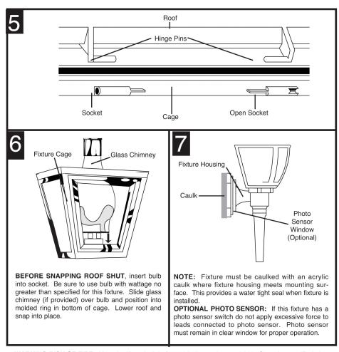
**WARNING-RISK OF FIRE.** Most dwellings built before 1985 have wire rated 60°. Consult a qualified electrician before installing. If supply wires are located within three inches of ballast, use wire rated for at least 90°C.
