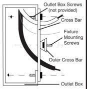
**THREAD** fixture mounting screws (provided) into outer cross bar.
