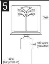
POSITION THE FIXTURE over the post as shown. For permanent mounting, fasten with set screw at hole in post collar by drilling hole at same location through post and securing with screw.
