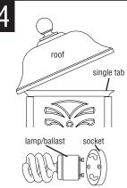
INSTALL integrated lamp/ballast. Use integrated lamp/ballast as specified on fixture. Grasp the plastic base, insert the pins into the socket and rotate clockwise until secure.
