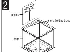
INSTALL PLASTIC PANELS, beginning with the panel under the roof hinge area, by sliding panel down cage in slot on inside of cage. Make sure panel is all the way down seated into cage. Tilt panel until top is resting next to lens holding block. Lift lens holding block up away from lens edge and then snap lens into place behind lens holding block.
