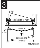
ATTACH FIXTURE ROOF TO FIXTURE CAGE. Squeeze cage as shown. Position holes on side of cage over corresponding pins on underside of roof. Release cage - pins will snap into position.
