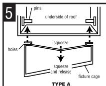
ATTACH THE FIXTURE ROOF TO FIXTURE CAGE. Squeeze cage as shown. Position holes on side of cage over corresponding pins on underside of roof. Release cage -
