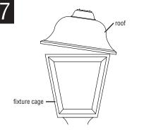
SCREW LIGHT BULB INTO SOCKET. Be sure to use bulb with wattage no greater than specified for this fixture. Lower roof and snap into place.
