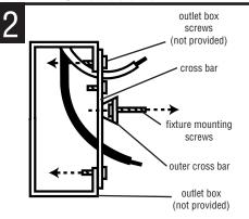
THREAD the fixture mounting screws (provided) into the outer cross bar.
