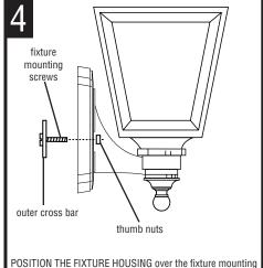
screws and secure in place with the thumb nuts provided.
