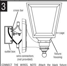
CONNECT THE WIRES. NOTE: Attach the black fixture wire to the black supply wire, the white fixture wire to the white supply wire. Do not mix them up. Use approved wire connectors (not provided).
