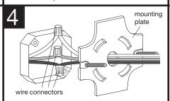
CONNECT THE WIRES. NOTE: Attach black fixture wire to black supply wire, white fixture wire to white supply wire. Do not mix them up. Use approved wire connectors (not provided). Connect bare fixture ground wire to ground wire from outlet box. NEVER CONNECT GROUND WIRE TO BLACK OR WHITE POWER SUPPLY WIRES.
