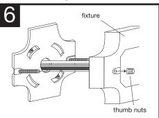
Position fixture over fixture mounting screws and secure with provided thumb nuts.
