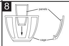
INSTALL PLASTIC PANELS, beveled side out, by sliding panels down cage in slots on inside of cage. Make sure panels are all the way down into seats in cage.
