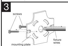
Thread one inch long screws into mounting plate and feed fixture wires through the hole in the center of the mounting plate.
