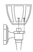
FASTEN THE CAGE to the fixture base with the three screws provided.
