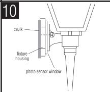
NOTE: Fixture MUST be caulked with an acrylic caulk where fixture housing meets mounting surface. This provides a water tight seal when fixture is installed.
