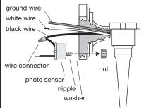
PLACE RUBBER WASHER over threaded nipple. Insert nipple through hole in fixture base. Thread nut onto nipple. Connect black wire from fixture to one of the black wires from photo sensor with wire connector provided.
