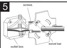
Attach swivel bar to outlet box with two 8-32 screws (not provided). These screws inserted through appropriate rectangular opening in plate and into swivel bat. Tighten screws.
