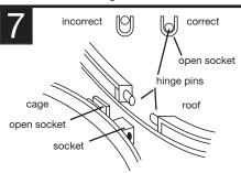
SLIP ONE HINGE PIN on roof into hole in socket on cage and snap other hinge pin into open socket. Be sure hinge pin is completely seated in open socket.
