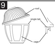
SCREW LIGHT BULB INTO SOCKET. Be sure to use bulb with wattage no greater than specified for this fixture. Lower roof and snap into place. See assembly illustration.
