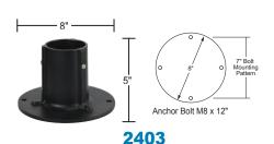
Die Cast Aluminum Flange base, Powdercoated Finish Anchor Bolts Included, for 8' -12' x 2.950" O.D. Posts only SPECIFY: Black, (B) Bronze, or (W) White
