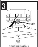
POSITION THE FIXTURE BASE over the nipple and secure into place with the fixture mounting knob.
