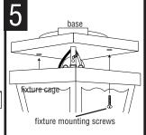
SCREW LIGHT BULB(S) INTO SOCKET. Be sure to use bulb with wattage no greater than specified for this fixture. Align holes in cage with holes in base and secure with fixture mounting screws provided.
