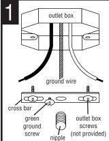
ATTACH CROSS BAR to outlet box with outlet box screws (not provided). THREAD NIPPLE into cross bar. Adjust nipple to proper height for mounting fixture
