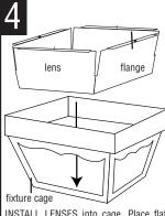
INSTALL LENSES into cage. Place flat lens in bottom and insert four side lenses as shown.
