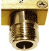
A photograph of an N Female RF connector. It is a brass-colored metal component with a threaded section and a central hole for a pin to fit into.      |
