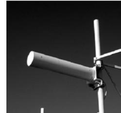
The CTI 5636 14dBi Yagi Antenna (pictured right) is a very powerful, highly directional antenna, and is capable of significant range when installed correctly.
