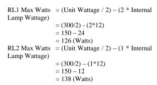
Ensure total unit load (including internal lamps) does not exceed unit rating including internal lamp loads.
