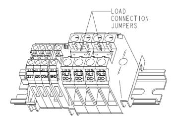
1. A terminal block for the remote lamp loads is provided for easy installation. Two terminals are available for DC+ and DC-each. Units ship from the factory with load connection jumpers installed on both DC+ and DC-. This parallels the load among the unit RL1+ and RL2+ output load fuses. Using the jumpers ensures that the total load of the unit is evenly distributed.
