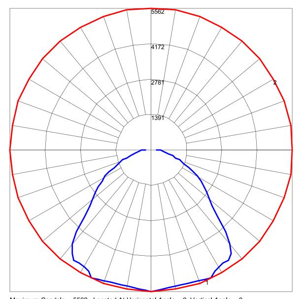
Maximum Candela = 5562 Located At Horizontal Angle = 0, Vertical Angle = 0 # 1 - Vertical Plane Through Horizontal Angles (0 - 180) (Through Max. Cd.) # 2 - Horizontal Cone Through Vertical Angle (0) (Through Max. Cd.)
