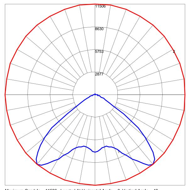
Maximum Candela = 11506 Located At Horizontal Angle = 0, Vertical Angle = 40 # 1 - Vertical Plane Through Horizontal Angles (0 - 180) (Through Max. Cd.) # 2 - Horizontal Cone Through Vertical Angle (40) (Through Max. Cd.)
