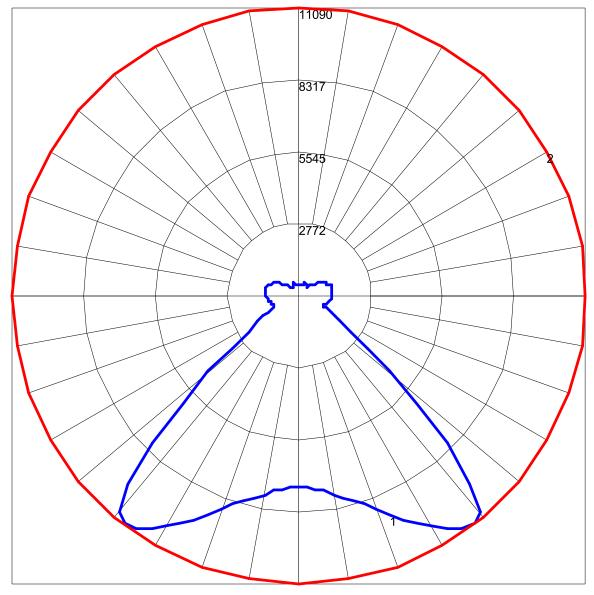
Maximum Candela = 11089.67 Located At Horizontal Angle = 0, Vertical Angle = 37.5 # 1 - Vertical Plane Through Horizontal Angles (0 - 180) (Through Max. Cd.) # 2 - Horizontal Cone Through Vertical Angle (37.5) (Through Max. Cd.)
