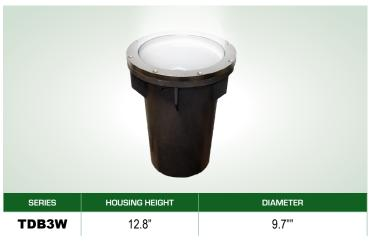
**MOUNTING** — Fixtures are designed to be in-ground burial lights and should be installed according to the installation instructions made available by Techlight. Proper drainage and substrate must be provided for water to flow freely through the well sleeve. A ¾" conduit entry is supplied into the anti-siphon chamber of the housing. Conrete pour kits available (see Accessories).
