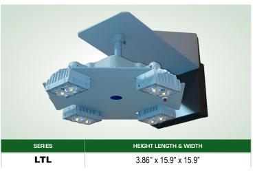
25°C ambient temperature at 1400mA operation. Lumen Maintenance >99% at 60K hrs. Optional 0-10V dimming. Built-in surge protection up to 10 kV. Built-in Active PFC Function >95%/Full load. LED Power Supply conforms to UL1310 Class 2 and UL8750 standards and is IP67 rated for wet locations
