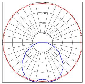
Maximum Candela = 4197.178 Located At Horizontal Angle = 50, Vertical Angle = 13 # 1 - Vertical Plane Through Horizontal Angles (50 - 230) (Through Max. Cd.) # 2 - Horizontal Cone Through Vertical Angle (13) (Through Max. Cd.)
