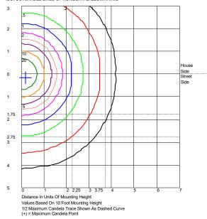
IES INDOOR REPORT PHOTOMETRIC FILE NAME: CSL S N90 DL 1 POLAR GRAPH 96W LED Canopy / Soffit Color Temperature: 4,000 K CRI: 90
