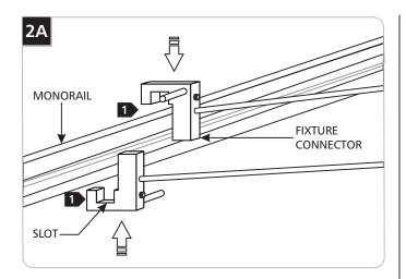
1 Place one fixture connector slot from the top and the other one from the bottom onto the MonoRail.
