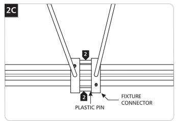
2 Slide the fixture connectors toward each other so that the plastic pins on the fixture connector slips into the side hole on the opposite fixture connector.
