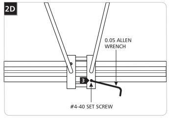
Tighten the #4-40 set screws on the fixture connectors with the 0.05 Allen wrench.
