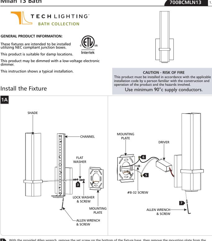
With the provided Allen wrench, remove the set screw on the bottom of the fixture base, then remove the mounting plate from the fixture base
