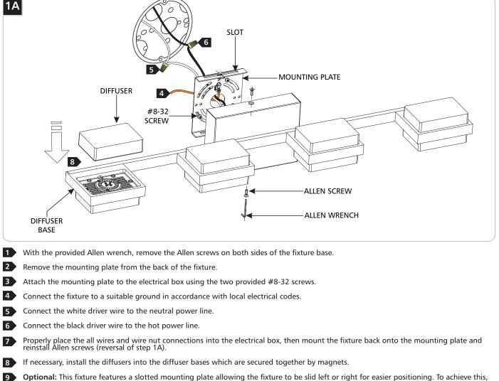
**Optional:** This fixture features a slotted mounting plate allowing the fixture to be slid left or right for easier positioning. To achieve this, loosen the Allen screws with the provided Allen wrench, slide the fixture base left or right until the desired position is reached, and retighten the Allen screws to secure in place.
