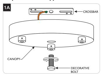
1 Remove the crossbar from the canopy by completely unscrewing the decorative bolt.
