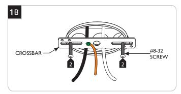
2 Mount the crossbar assembly to the electrical box with the two provided #8-32 screws.
