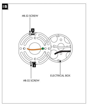
**3** Install the mounting plate onto the electrical box with the two #8-32 screws provided.
