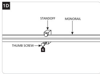
6 Place the MonoRail into the standoff slot. Use the thumb screws to secure the MonoRail to the standoffs.
