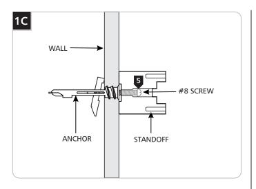
**5** Screw the standoff onto the anchor with the #8 screw.
