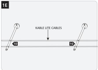
**10** Feed the Kable Lite cables coming from the turnbuckles through the standoff holes.
