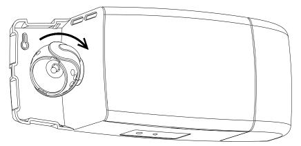
LAMP HEAD AIMING – Remove lens covers as shown in step 1. Lamp heads may be aimed by grasping them at the base and rotating them to aim at the desired location. Lamp head only rotates approximately 135° which is enough to aim in any direction whether mounted on wall or ceiling.
