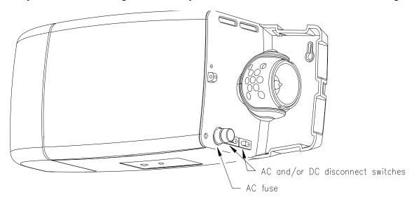
AC FUSE AND AC OR DC DISCONNECT SWITCH OPTIONS - If ordered, these options can be found under the right lamp head lens.
