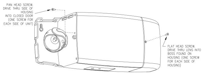
TAMPERPROOFING - If ordered, install this option using the included screw kit which includes two flat head screws, two pan head screws and a tamperproof Torx T-15 bit.
