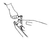
SLIDE UNIT ONTO THE PIPE MOUNTING ARM UNTIL END OF PIPE RESTS ON "LEVELING STEPS". CARE IS TO BE TAKEN SO ARM DOES NOT INADVERTANTLY STRIKES BALLAST.
