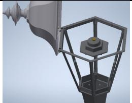
**Step 2:** Unfasten the retaining screw and open the fixture roof. Remove any existing optics in the roof and dispose of properly. Remove (2) screws and detach the fitter cap. Save the screws for later use in Step 3. Disconnect the supply lines and remove any attached ballast components from the fitter area. These components will not be required for this conversion.
