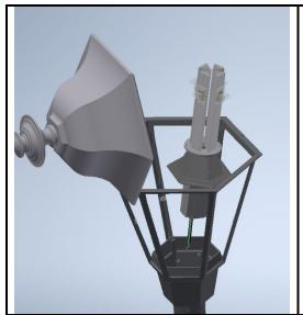
**Step 3:** Place VCOB in fixture and connect the supply lines to per wiring schematic. With the "STREET" designation on the fitter cap on the street side of the fixture, guide the cap in place, taking care not to pinch any wires between the cap and the fitter. Fasten the fitter cap in place with the screws from Step 2. Replace roof and fasten in place.
