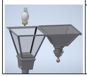
**Step 3:** Unlatch roof assembly and rotate to open position. Remove any optics in roof, and any lamps, sockets, or decorative chimneys on the fitter cap. These components will not be used for the retrofit.
