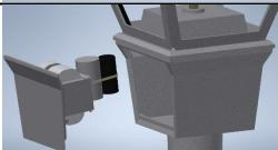
**Step 2:** Remove the fitter door and set it aside for later use. Disconnect supply lines from ballast. Remove ballast components and dispose of them properly.
