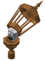
**Step 2:** Loosen the ballast retaining screw and lean the hinged cage assembly back. Disconnect supply lines from ballast. Remove ballast components and dispose of them properly. Carefully unfasten any optic components so they may be removed in the next step. Return roof to closed position and tighten the ballast retaining screw.
