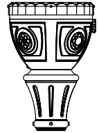
990 or 990T* Fits 3" OD x 3" tall tenon/pole 994 or 994T* Fits 4" OD x 3" tall tenon/pole
