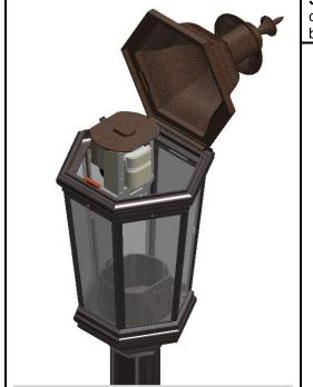
**Step 2:** Open the fixture and remove any existing optics. Unlatch the fitter cap and remove the cap and attached ballast. These components will not be required for this conversion. Discard/Recycle them per local code.
