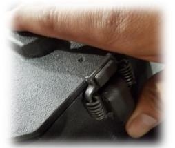
**Step 4:** With the "STREET" designation on the fitter cap on the street side of the fixture, latch cap in place, taking care not to pinch any wires between the cap and the fitter. Close and latch door.
