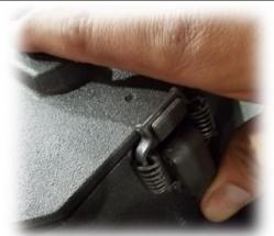
**Step 4:** Orient the "STREET" designation on the fitter cap to the street side of the fixture, and latch cap in place, taking care not to pinch any wires between the cap and the fitter. Close and latch door.
