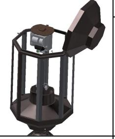
**Step 2:** Open the fixture roof and remove any existing optics. Unlatch the fitter cap and remove the cap and attached ballast. These components will not be required for this conversion. Discard/Recycle them per local code.
