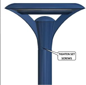
**STEP 5:** Uniformly tighten all 3 set screws located at the bottom of the fixture to secure the fixture to the Tenon.
