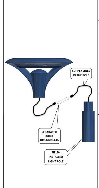
**STEP 1:** Disconnect the male quick disconnect from the female quick disconnect.
