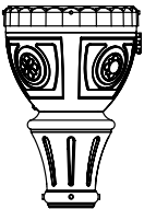
990 Fits 3" OD x 3" tall tenon/pole 994 Fits 4" OD x 3" tall tenon/pole
