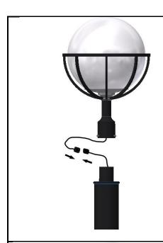
**Step 1:** Disconnect male the quick disconnect from the female quick disconnect.
