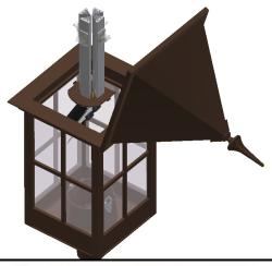
**Step 3:** Place VCOB in fixture and connect the supply lines to per wiring schematic.
