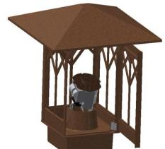
**Step 2:** Open the fixture door and remove any existing optics. Unlatch the fitter cap and remove the cap and ballast assembly These components will not be required for this conversion.
