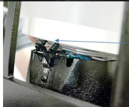
**Step 6:** Lift the VCOB unit slightly and lift the hinged clamp bar over the hook on the cover on one side of the unit. Repeat for other side.
