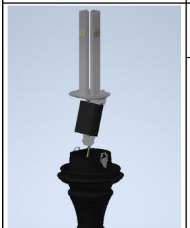
**Step 4:** Connect the VCOB retrofit kit to the supply lines. With the "STREET" designation on the fitter cover on the street side of the fixture, place the cover on the fitter taking care not to pinch any wires between the cap and the fitter. Latch the cover in place. Replace globe and tighten set screws uniformly.
