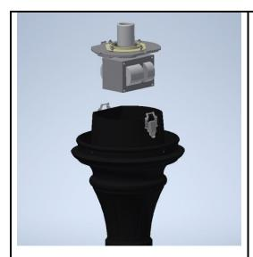
**Step 3:** Unlatch the two latches on the fitter cover and lift it out of the fitter. Disconnect the supply wiring from the ballast. These components will not be needed for the retrofit. Please dispose of the cover and ballast assembly properly.
