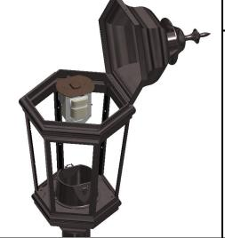
**Step 2:** Open the fixture roof and remove any existing optics. Unlatch the fitter cap and remove the cap and attached ballast. These components will not be required for this conversion. Discard/Recycle them per local code.
