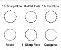
All Tapered Shafts have a taper of 0.14 inch per foot of length, most shafts are available in steel and/or aluminum.
