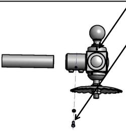
**Step 1:** Loosen but do not remove the (3) 1/4-20 Set Screws in Cap. **Step 2:** Remove the Cap from Hang Straight Fitter Box. If supplied with a Finial or Photocell do not remove them from the Cap. Disconnect Photocell
