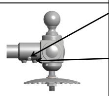
**Step 10:** Apply Loctite® Red Threadlocker or equivalent to the threads and install the 3/8-16 X 1-1/4" Hang Straight Safety Bolt with 3/8" Hex Lock Nut fully against the bolt head into the tapped hole on the side.
