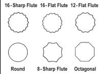
All Tapered Shafts have a taper of 0.14 inch per foot of length, most shafts are available in steel and/or aluminum.
