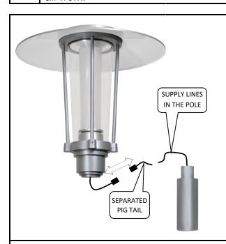
**Step 1:** Disconnect the male quick disconnect from the female quick disconnect.
