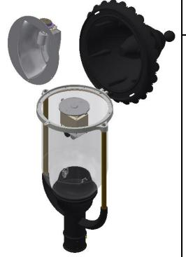
**Step 2:** Open the fixture roof and remove any existing optics. Remove the fitter cap screws, lift the cap, and disconnect the supply lines. Remove the cap and attached ballast. These components will not be required for this conversion. Discard/Recycle them per local code.
