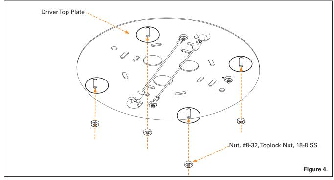
Step 2. Preload the Top lock nut to the Driver top plate. Figure 4
