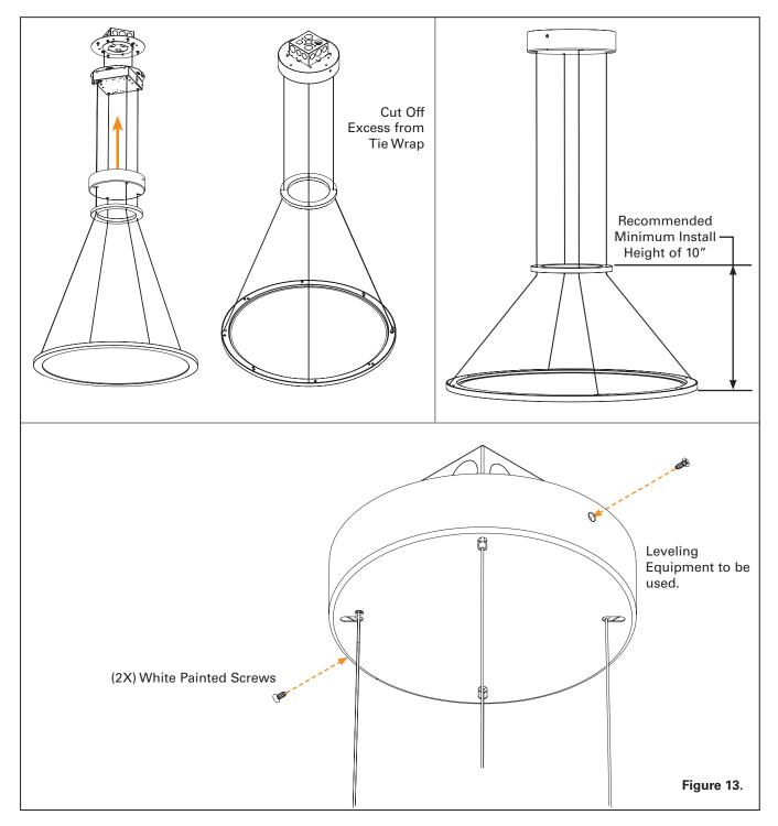
**Step 14**. Raise Decorative Cover and attach to the Driver Compartment using 2X M4 flat head screw (head painted white). Use Tie Wraps to keep the Low Voltage Cable taut against the Air Craft Cable. Figure 13
