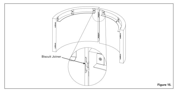
Step 15. Align and insert the biscuits from on adjacent panel to another. Figure 15Step 16. Use pressure to press downwards, and forcefully snap together. Figure 15Step 17. Attach all 4 acoustic Drum panels together to make a sub-assembly. Figure 15
