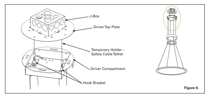
**Step 10.** Lift the entire fixture by holding the Driver Compartment and suspend the fixture with the cables from Driver Top Plate. Figure 9
