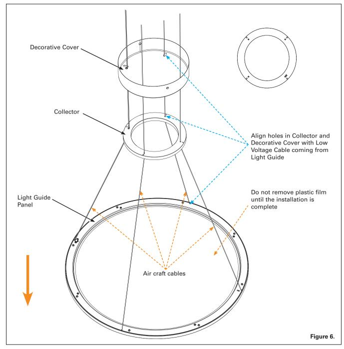
**Step 4** Take the four Air Craft Cables and Low Voltage Cables and feed them all the way through the Collector and Decorative Cover. Make sure to orientate the Collector and Decorative Cover so the Low Voltage Cable feeds through the correct features in the parts. The Low Voltage Cable will also need to orientate with the hole in the Driver Compartment Cover in the ceiling. Figure 6
