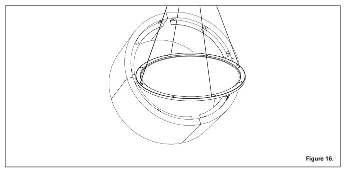
**Step 18.** Insert the Light Guide Panel in to the Acoustic Drum panel sub-assembly in the air through openings between curved bracket.
