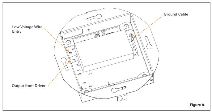
**Step 8**. Make the Low Voltage wire connections to the driver (LED output), with the Wire nuts provided. Figure 8 **Step 9**. Use the Ground Cable from driver box, to ground from J-Box wire and make connection with the wire nuts provided for ground. Figure 8
