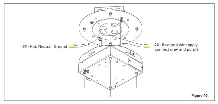
**Step 11.** Connect the wires (main line) coming from J- Box with the driver. Figure 10 (Reference – one more view is shown).
