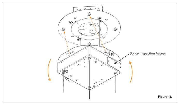
**Step 12**. Slightly rotate the fixture so that the Preloaded Nuts align with the Key slot. Push the entire fixture up holding the driver box and let the excess cables and wire pack inside the driver compartment. Figure 11
