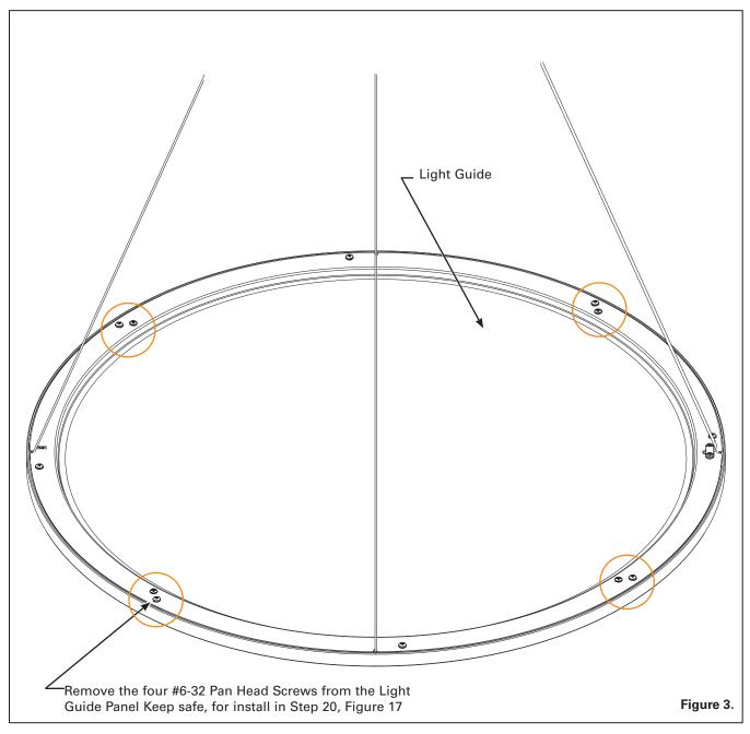
**Step 1.** The Following Step #, is for the Light Guide Panel with acoustic Drum panels. Complete this step before Light Fixture is hung. Figure 3
