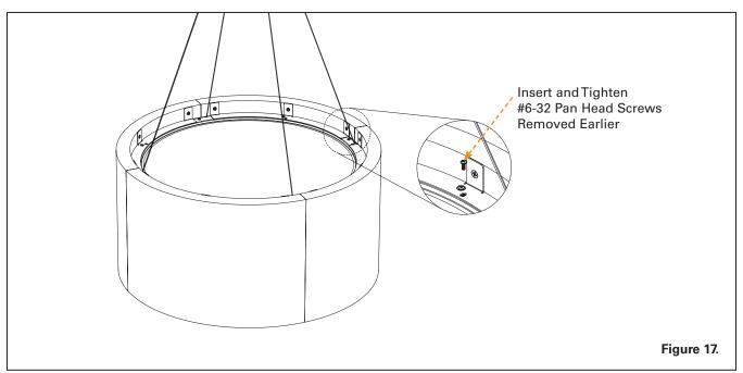
**Step 20**. Align all the 4 holes of the Acoustics brackets to the Light Guide Panel holes and fasten the screws that were removed before assembly of Light Guide Panel. Figure 17
