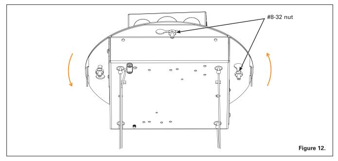
**Step 13**. Once the Key hole and #8-32 lock Nut has been oriented, slightly rotate the fixture so that the Stud slips into narrow portion of Keyhole. Once the position is fixed, tighten the nuts firmly (total 4 Nuts). Ensure all wires are inside driver enclosure and ensure no pinched wires. Figure 12
