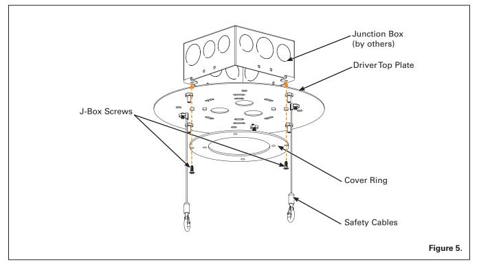
**Step 3**. Using the J-Box screws, align the Cover Ring to inside of the Driver Top Cover. Screw the cover ring and the driver top plates to the J-Box. The Cover Ring must be used to reinforce the center of the Top Plate. Figure 5
