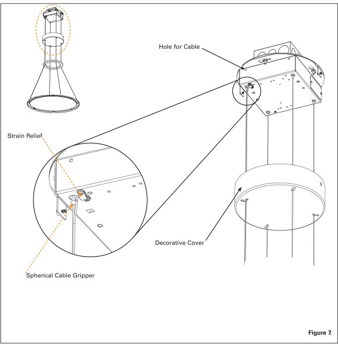
**Step 6.** Insert the Air Craft Cables into the spherical shape Cable Grippers in the Driver Compartment. Raise Light Guide Panel by continuing to feed the Air Craft Cables through the Grippers, pulling the excess cable out of the hole for air craft cable as the light fixture is raised. To lower the cables, gently push up on the neck of the Gripper. Figure 7
