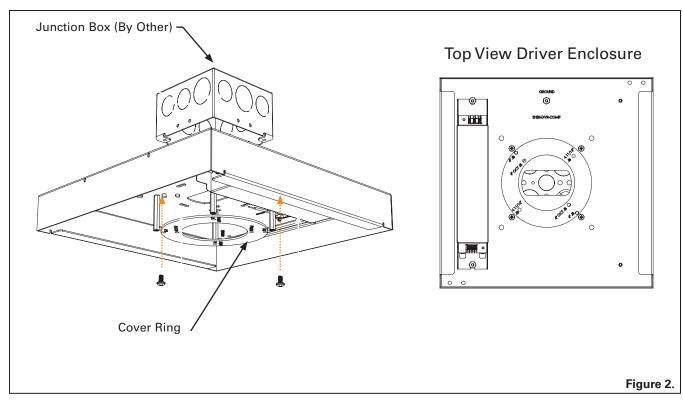
**Step 2.** Using the J-Box screws (by others), align the Cover Ring to inside of the Driver Compartment. Screw the parts to the J-Box. The Cover Ring must be used to reinforce the center of the housing. Ref. Figure 2.
