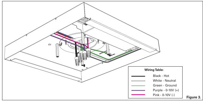
**Step 3.** Connect feeder wires from contractor supplied junction box to power wires of fixture using supplied wire nuts. Tuck all wires inside junction except blue and red low voltage wires (used for controls, and reference wiring diagram). Ref.Figure 3.
