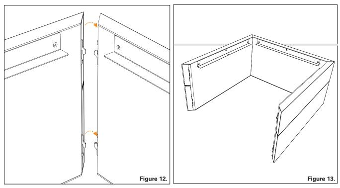
**Step 12 and 13.** Assemble three of the Acoustic Panels together on the ground ensuring the finger biscuits lock together. Ref. Figure 12 and 13.
