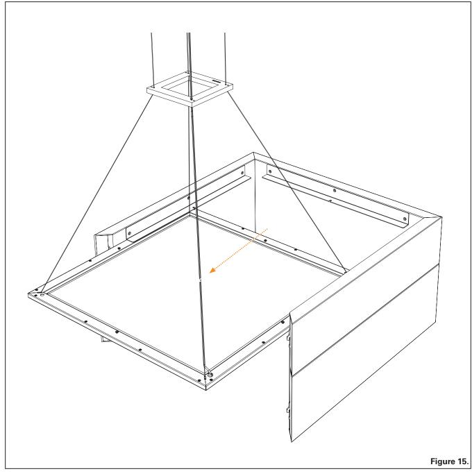
**Step 15**. Take the three Acoustic Panels and carefully slide them over the top of the Light Guide Panel and reinstall three of the #6-32 pan head screws through the acoustic panel brackets. Ref. Figure 15.
