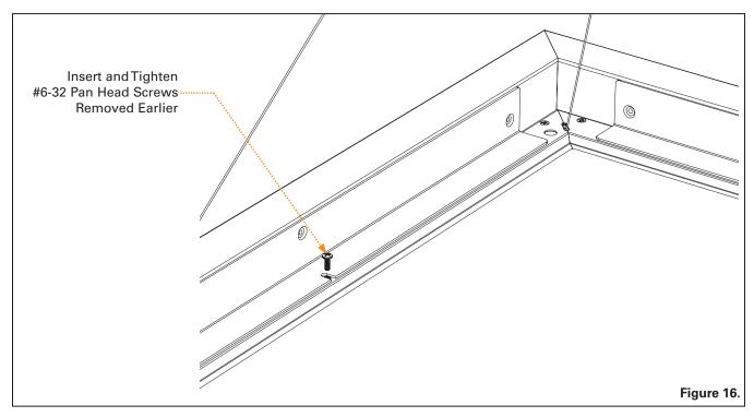
Step 16. Attach the last acoustic panel by locking the finger biscuits together. Use caution not to pull on the Light Guide Assembly and install the last #6-32 screw in the fourth Acoustic Panel bracket. Once install is complete, remove protective film and foam from light guide panel and acoustic panels.
