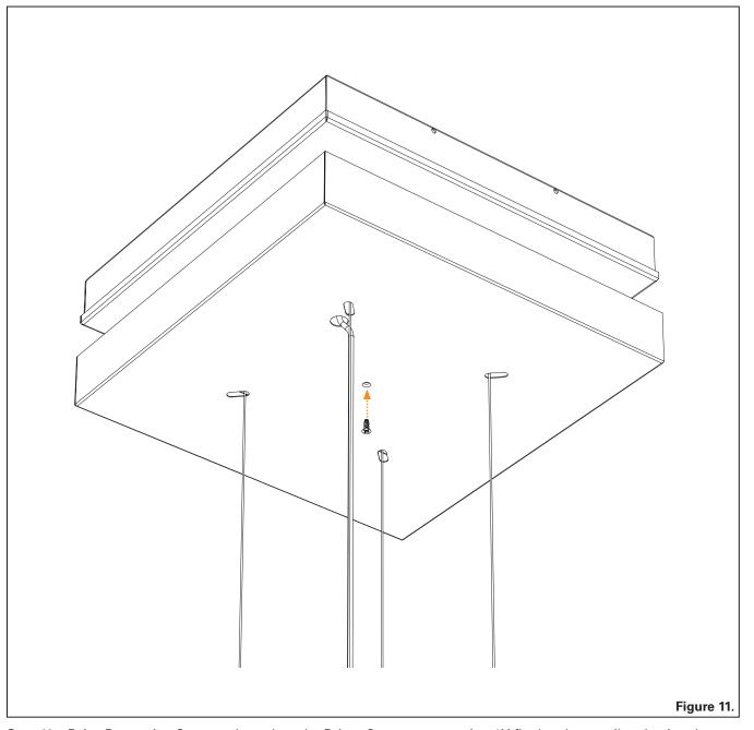
**Step 11a.** Raise Decorative Cover and attach to the Driver Compartment using 1X flat head screw (head painted white). Ref. Figure 11.
