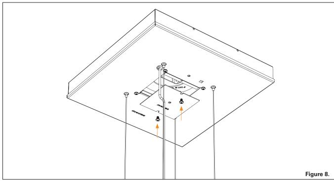
**Step 8.** When the final height is determined and leveling is complete, either cut the excess Air Craft Cable or tightly spool it up with a tie wrap. Wrap and tie excess low voltage wire and tuck into the Driver Compartment. Ref. Figure 8.
