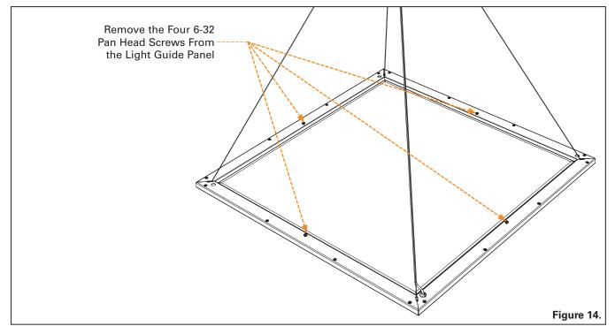
**Step 14**. Remove the four #6-32 pan head screws with white heads from the top of the Light Guide Panel. Ref. Figure 14.
