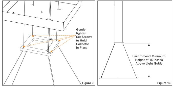
**Steps 9 and 10.** Once the Light Guide is at the approximate height raise up the Collector and Decorative Cover. Using the provided Hex L Key, gently tighten the set screws in the Collector secure it in the desired location. The Decorative Cover will rest on top of the Collector until the finial leveling of the Light Guide Panel with Air Craft Cables. Ref. Figures 9 and 10.
