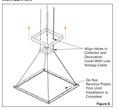
**Step 6a**. At the Light Guide Panel, take the four Air Craft Cables and Low Voltage Cable, feed them all the way through the Collector and Decorative Cover. Make sure to orientate the Collector and Decorative Cover so the Low Voltage Cable feeds through the correct features in the parts. The Low Voltage Cable will also need to orientate with the hole in the Driver Compartment Cover in the ceiling. Ref. Figure 6.
