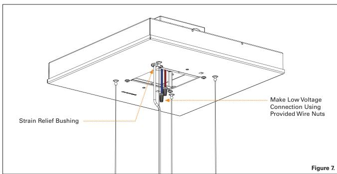
**Step 7.** Insert the Air Craft Cables into the spherical shape Cable Grippers in the Cover of the Driver Compartment. Raise Light Guide Panel by continuing to feed the Air Craft Cables through the Grippers, pulling the excess cable out of the Access opening as the light fixture is raised. To lower the cables, gently push up on the neck of the Gripper. Ref. Figure 7.
