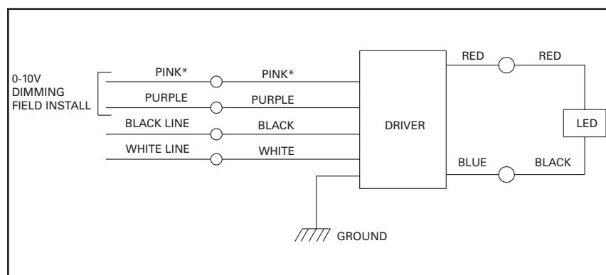
\* Constructions built before Jan 2022 may have gray wire for 0-10 dimming control present. In these cases, the installer will label the gray building wire as a 0-10 dimming wire and connect to our product's pink 0-10V dimming control wire. Reference NFPA70 (2020 NEC), section 410.69.
