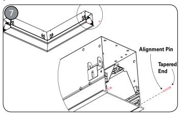
FOR CORNER INSTALLATION: Prepare corner unit for installation. Identify power feed side (end toward Beginning of Run). Prep wires on power feed side for connection to previous section in the run / pattern. Install alignment pins into extrusion non-power feed side using a hammer. Tapered side should face outward.
