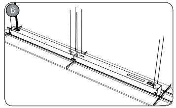
FOR CONTINUOUS RUNS: Secure next fixture in row using support wires on both sides of fixture. OPTIONAL STEP: Secure fixture to grid using #8 screws through grid bracket. Required for seismic installations. Repeat steps 5-6 as necessary.
