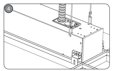
Secure fixture at both ends using support wire according to local building codes (not supplied).
