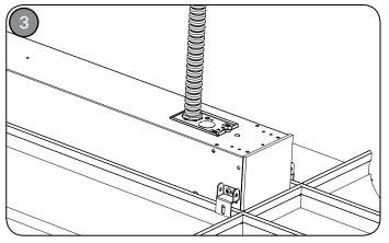
Reattach access plate by sliding plate back into housing as shown and secure access plate by re-installing screw.
