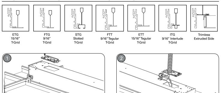
Prepare grid width spacing according to chart above and local building code. Install fixture housing into grid. Ensure Grid brackets secure over grid and fixture is resting on grid tee. Unscrew access plate and slide to remove as shown.
